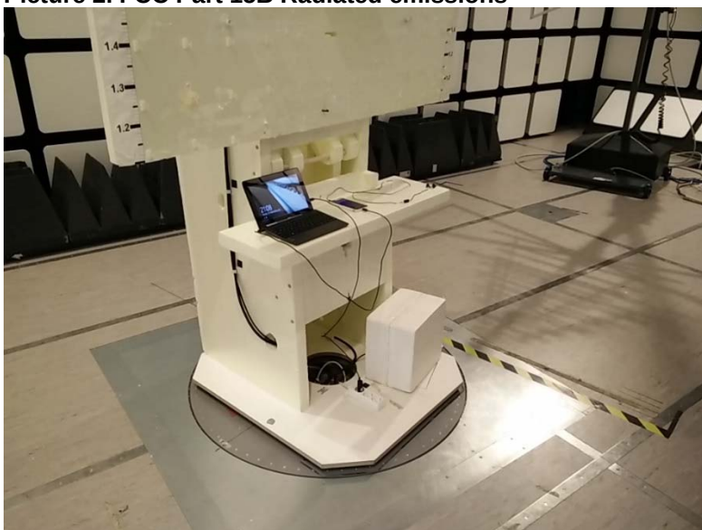
Picture 2. FCC Part 15B Radiated emissions
