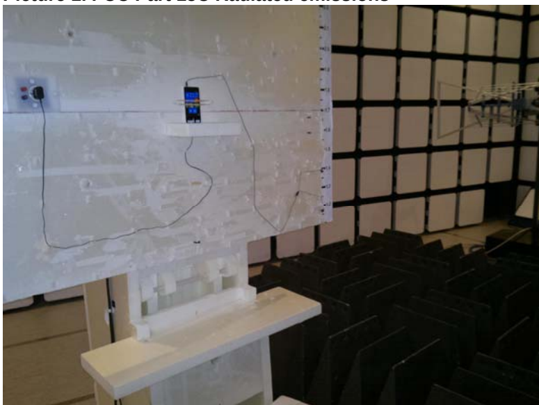
Picture 2. FCC Part 15B Radiated emissions
