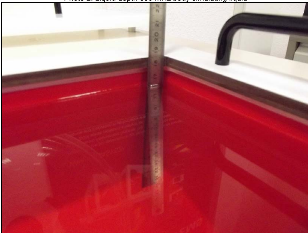
Photo 2: Liquid depth 850 MHz body simulating liquid
