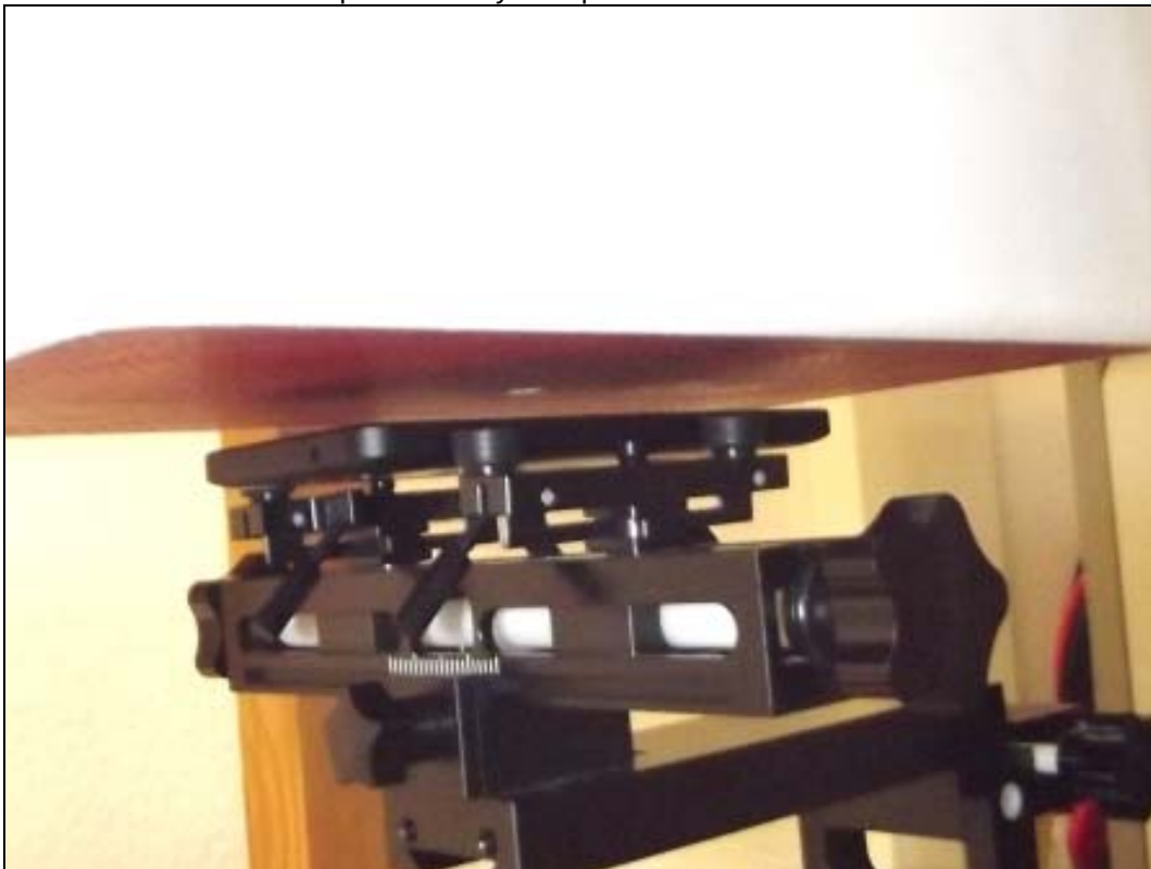
Photo 17: Test position body hot spot front side with 10 mm distance
