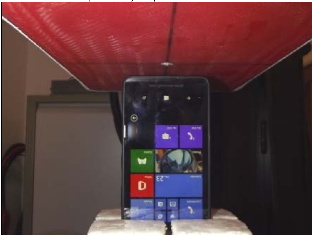
Photo 22: Test position body worn front side with 15 mm distance
