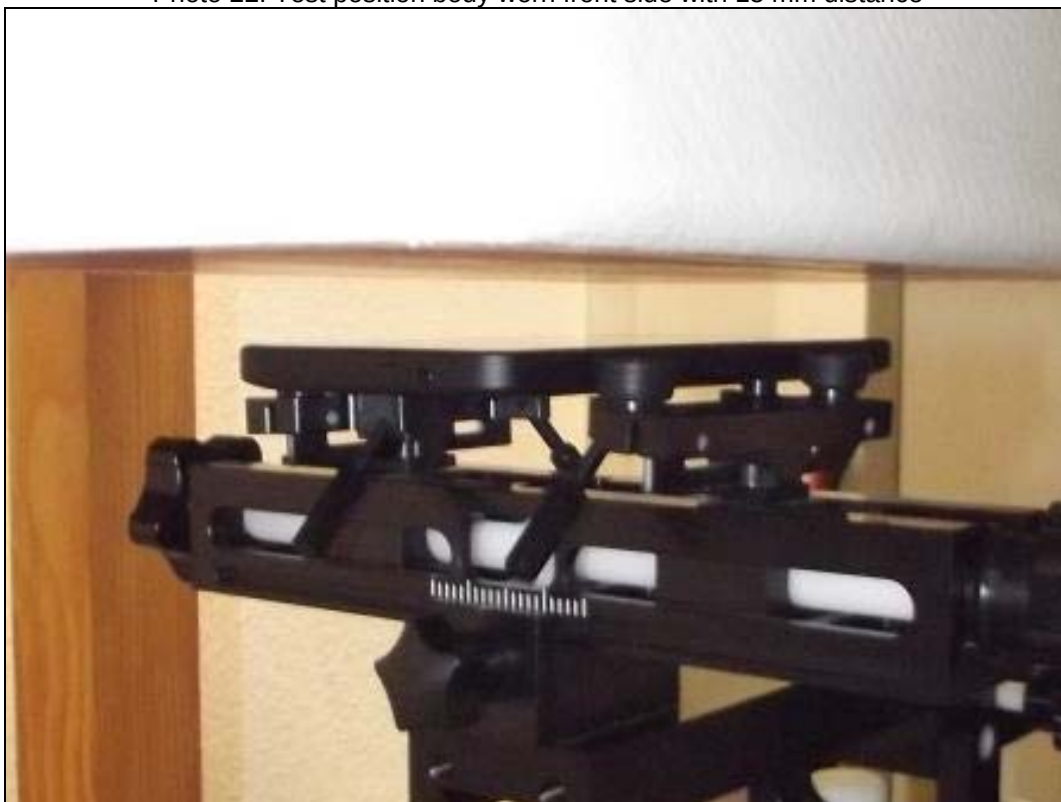
Photo 22: Test position body worn front side with 15 mm distance
