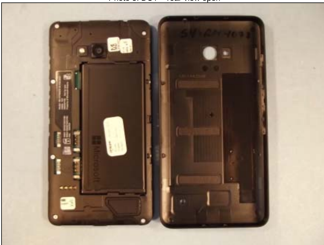
Photo 6: DUT – rear view open (without battery)
