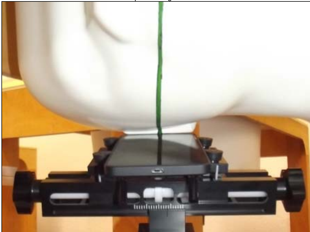
Photo 16: Test position right hand tilted 15°
