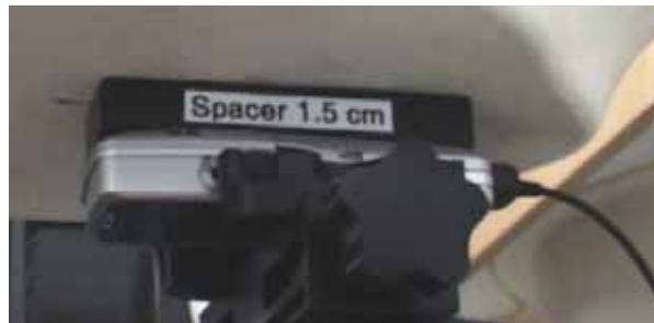
Photo of the device positioned for Body SAR measurement back side towards the phantom. The spacer was removed for the tests.
