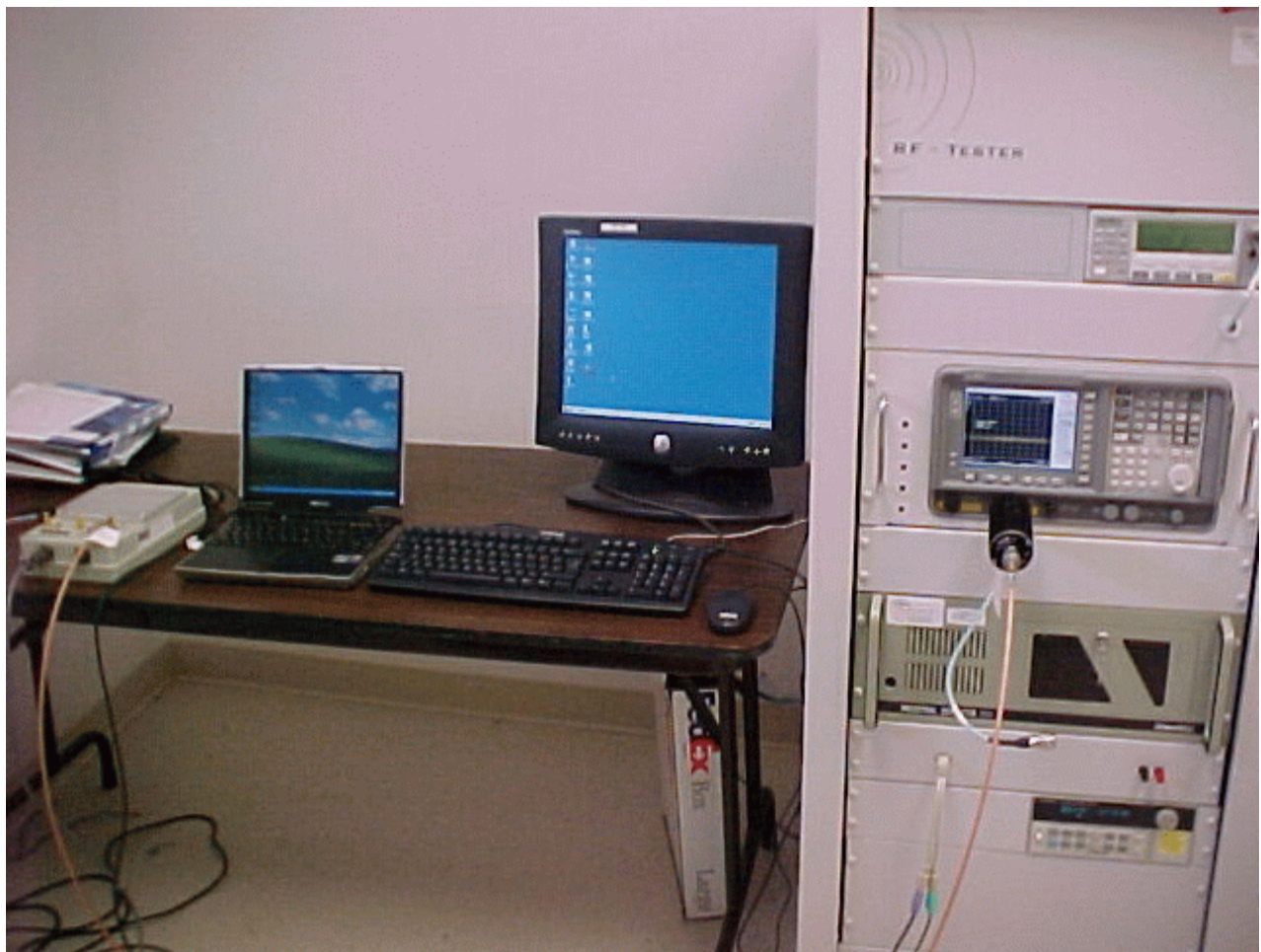
Photograph 1. RF Power Output Test Setup Photo
