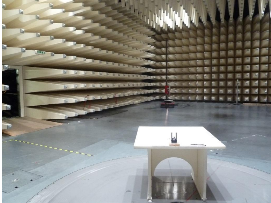
Photo 1 (RSE Setup 30 MHz to 1 GHz):
