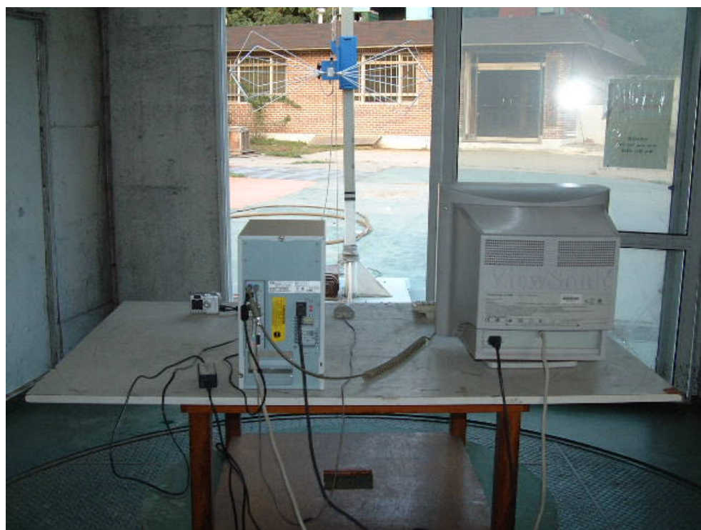
RADIATED EMISSION SETUP PHOTOGRAPH - REAR VIEW ( 30 - 300 MHz )
