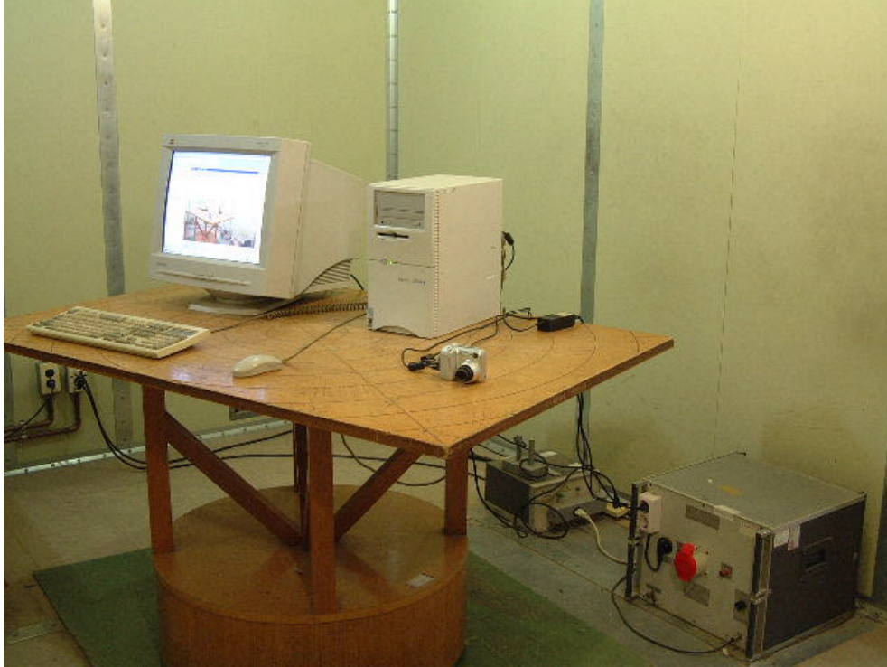
LINE CONDUCTED SETUP PHOTOGRAPH - FRONT VIEW
