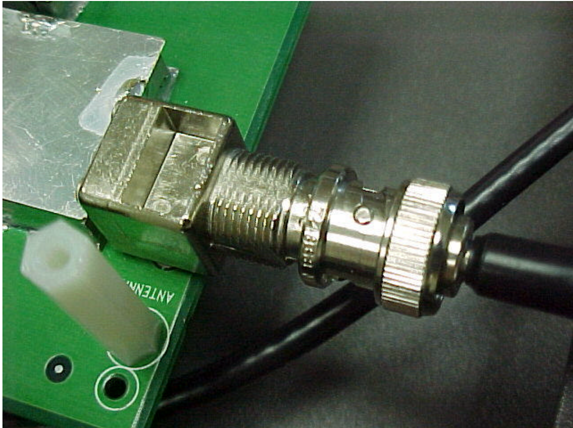
Photo Nine Single PCB showing Antenna Connection
