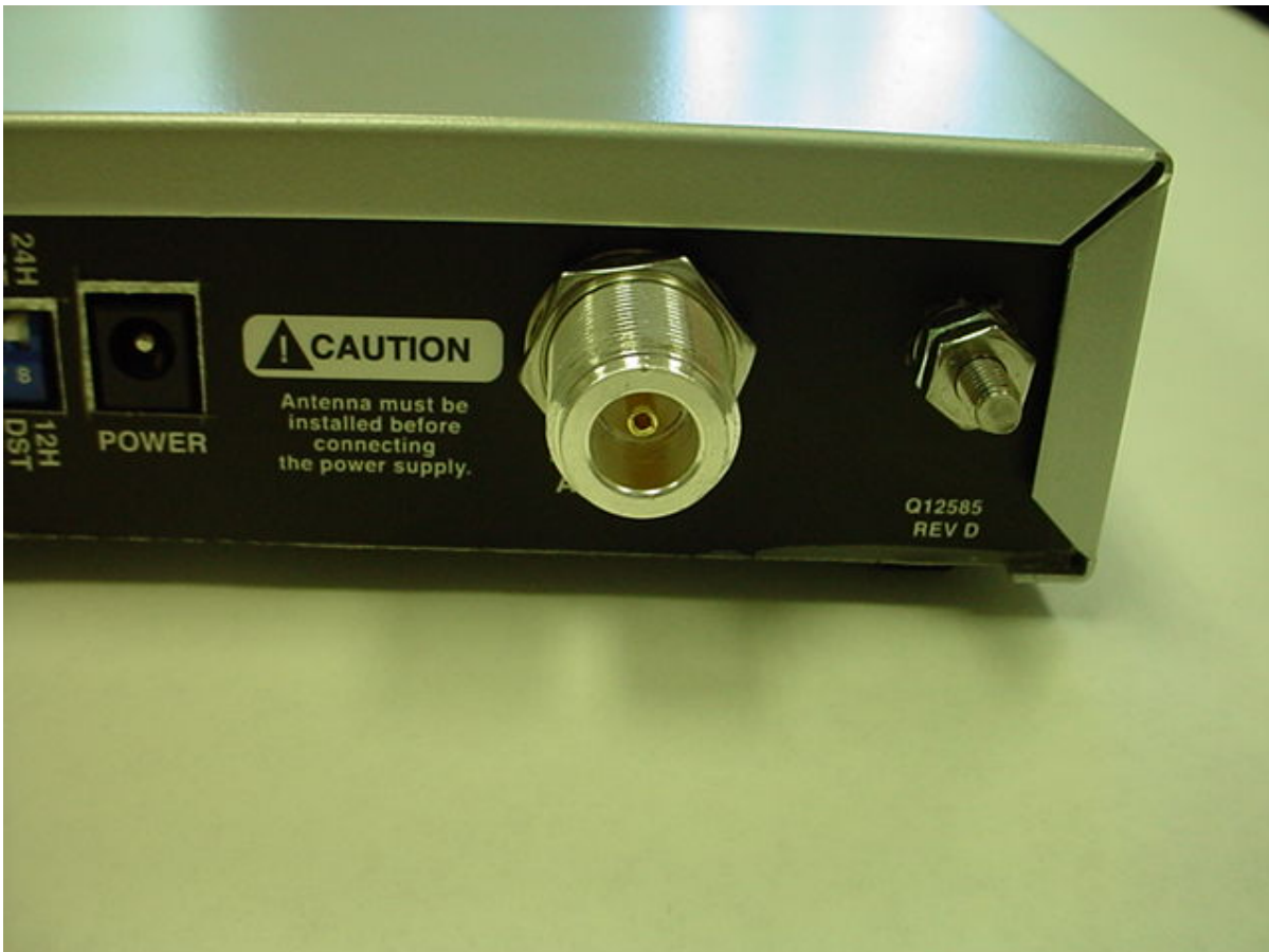
Photo Five – External Antenna Port
