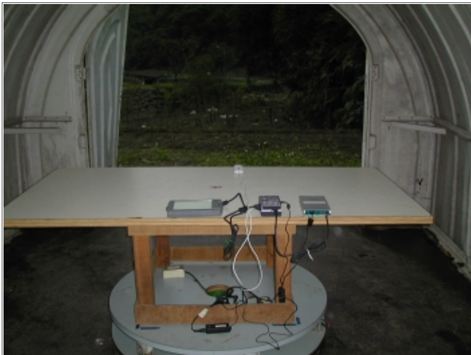
Radiated Emission Setup Photos (Worst Emission Position)
