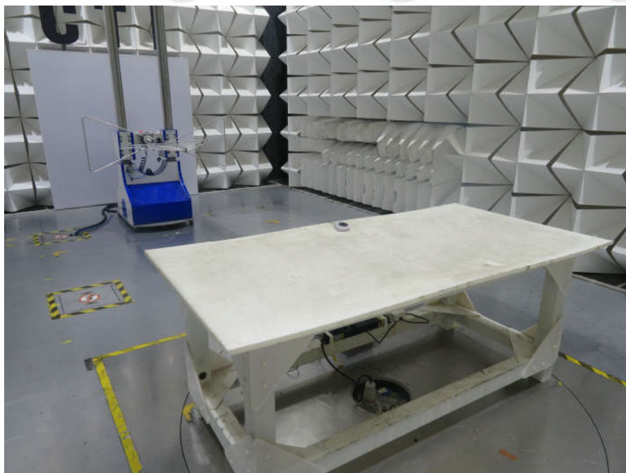
Radiated emission Test Setup-2(30MHz~1GHz)
