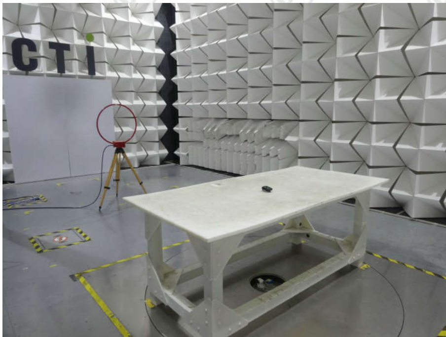
Radiated emission Test Setup-1(9kHz~30MHz)
