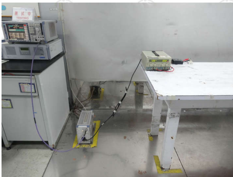
Conducted Emissions Test Setup
