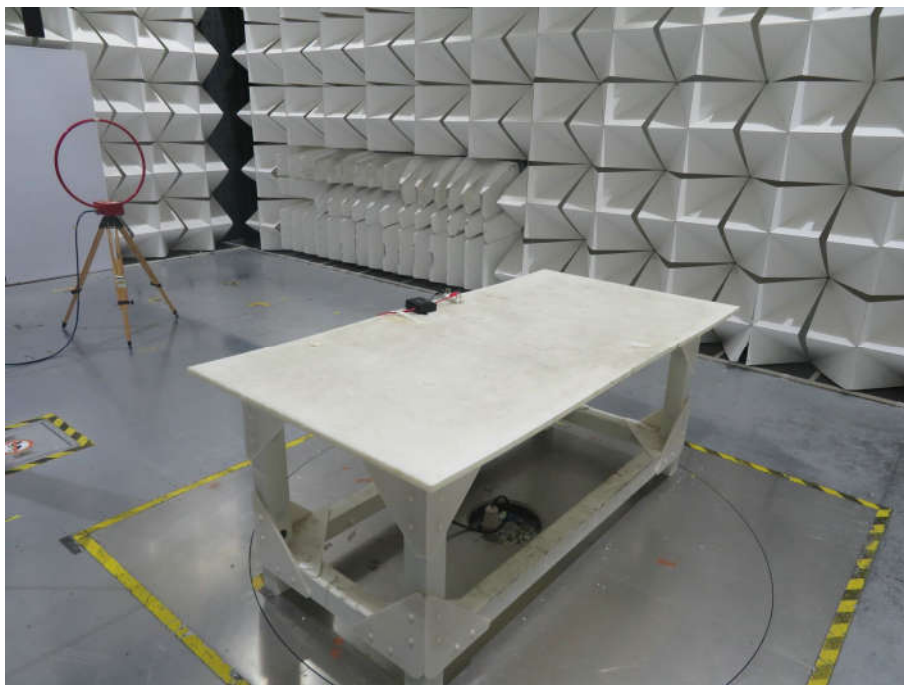
Radiated spurious emission Test Setup-1( 9K-30MHz )
