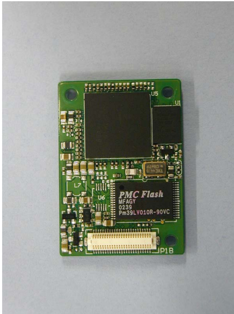
Component side of Wireless LAN
