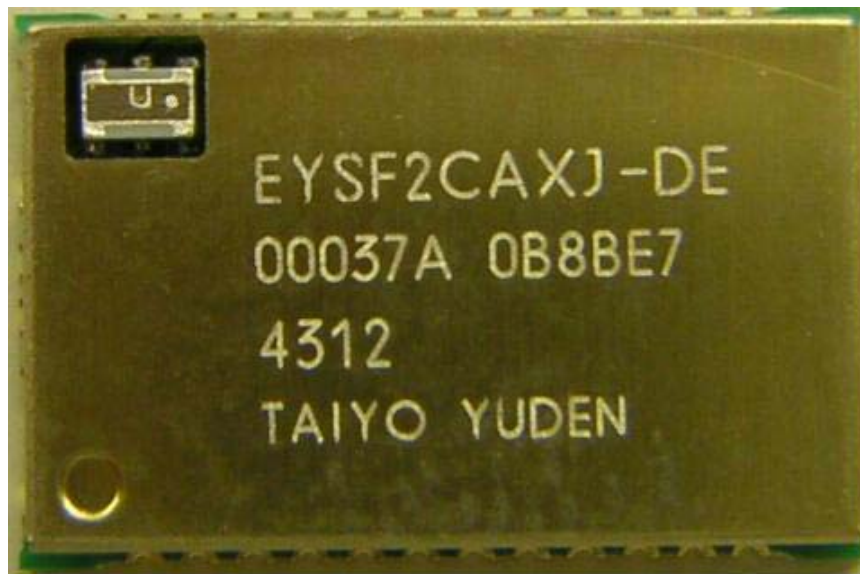
External Photo of Bluetooth Module IC (Component side)
