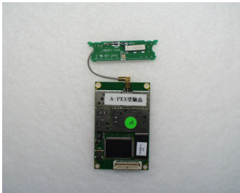
Back View of RF Module
