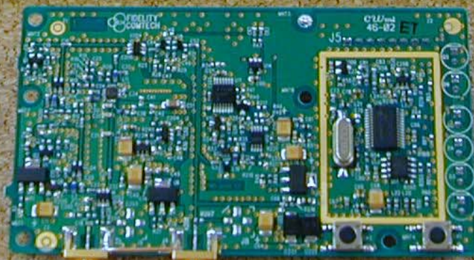
FCI-2451 Amplified Antenna (Witch's Hat) - Case Open - Amplifier Removed
