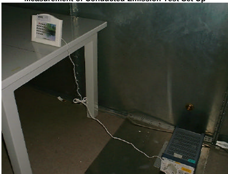
Measurement of Conducted Emission Test Set Up
