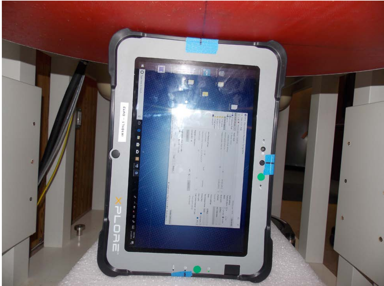
Test Configuration Left Side 0 mm Gap Photo from original testing for WiFi
