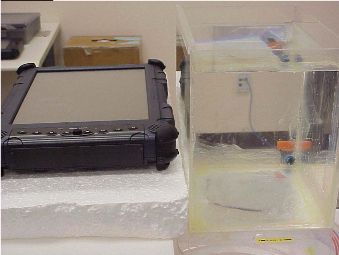
Photo 4. 2450 MHz antenna bystander position
