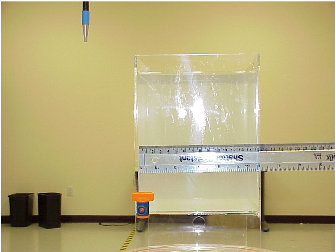
Photo 7. Photo to demonstrate 15 cm Z-axis flat phantom
