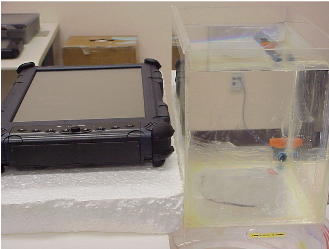
Photo 7. 2450 MHz antenna bystander position
