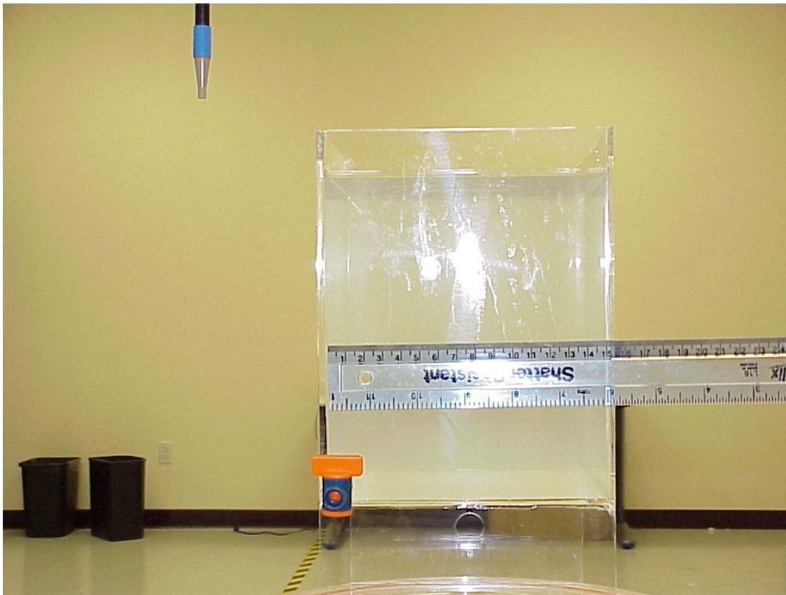
Photo 5 Photo to demonstrate 15 cm Z-axis flat phantom
