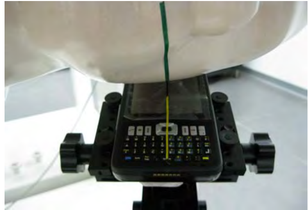
Fig.6 Left Head Section / Ear-Tilt Position(15°)
