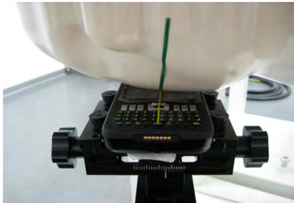
Fig.3 Right Head Section / Cheek-Touch Position
