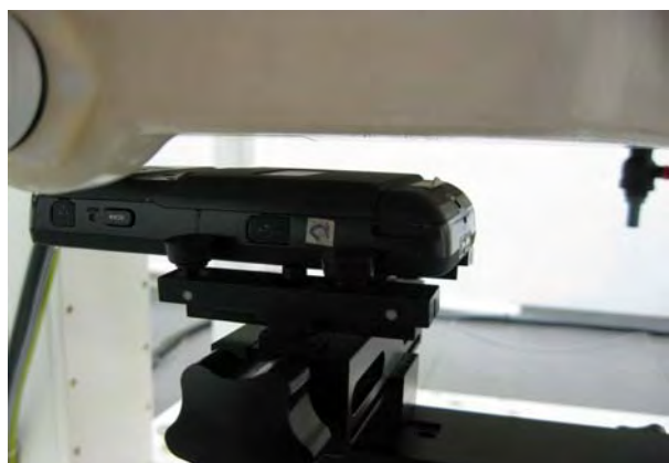
Fig.8 EUT back REID to flat phantom
