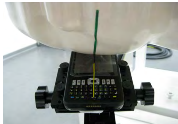
Fig.4 Right Head Section / Ear-Tilt Position(15°)
