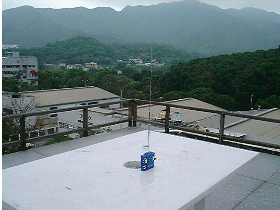
Measurement of Radiated Emission Test Set Up
