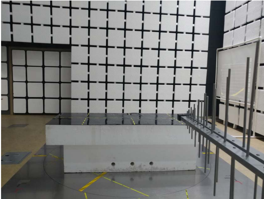
Radiated RF measurement (<1GHz) Left/Right ear
