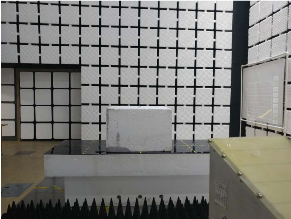
Radiated RF measurement (>1GHz) Right ear
