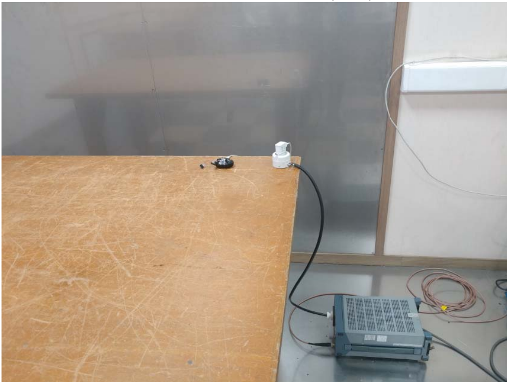
AC Conducted measurement (Front)
