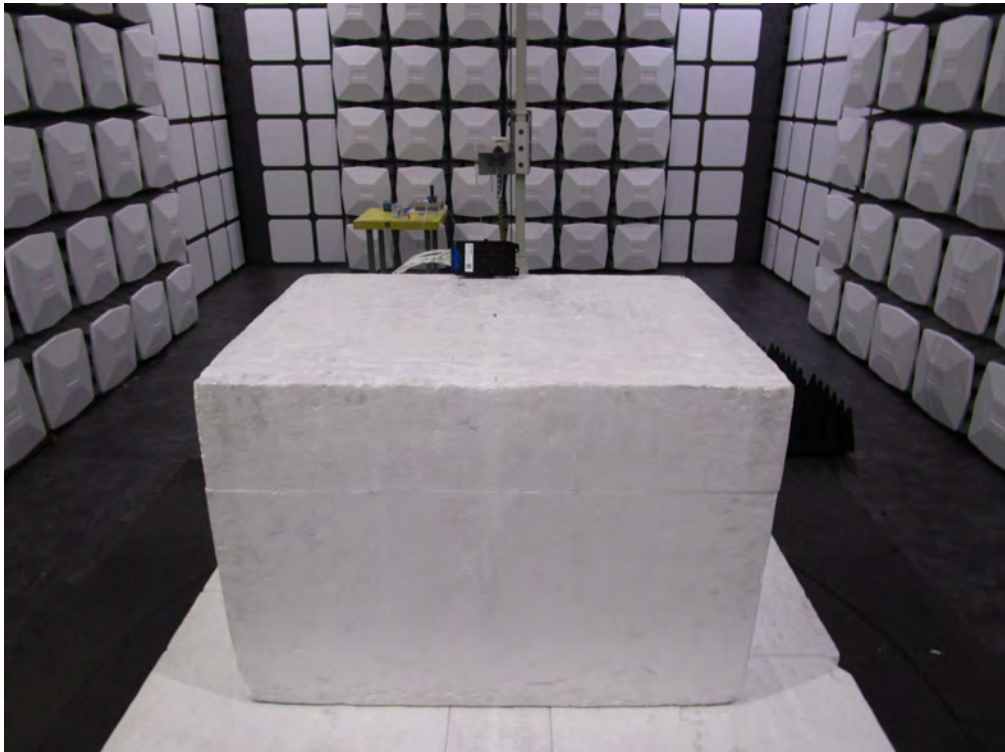
Description: Back View of Radiated Spurious Emission Test Setup (Above 1 GHz)
