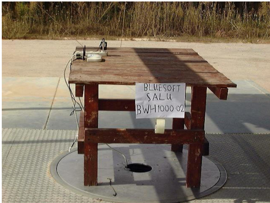
Figure 4. Spurious Radiated Emission Test Side (BWH1000-02)
