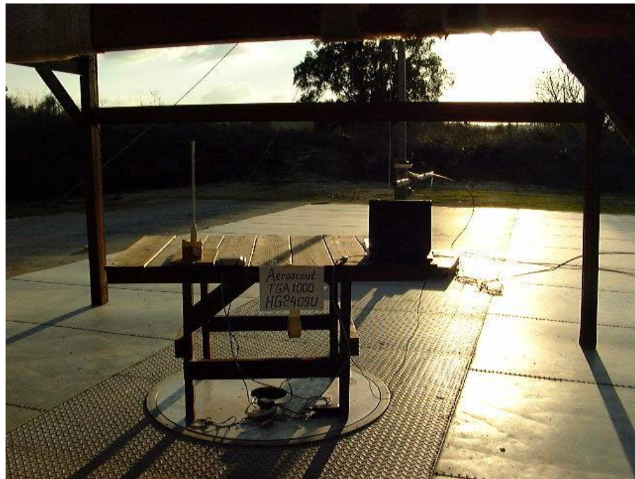
Figure 1. Spurious Radiated Emission Test Antenna HG2409U
