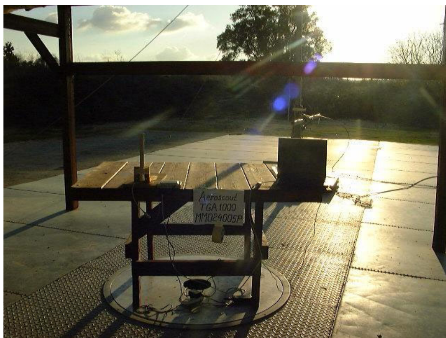
Figure 4. Spurious Radiated Emission Test Antenna MM024005P
