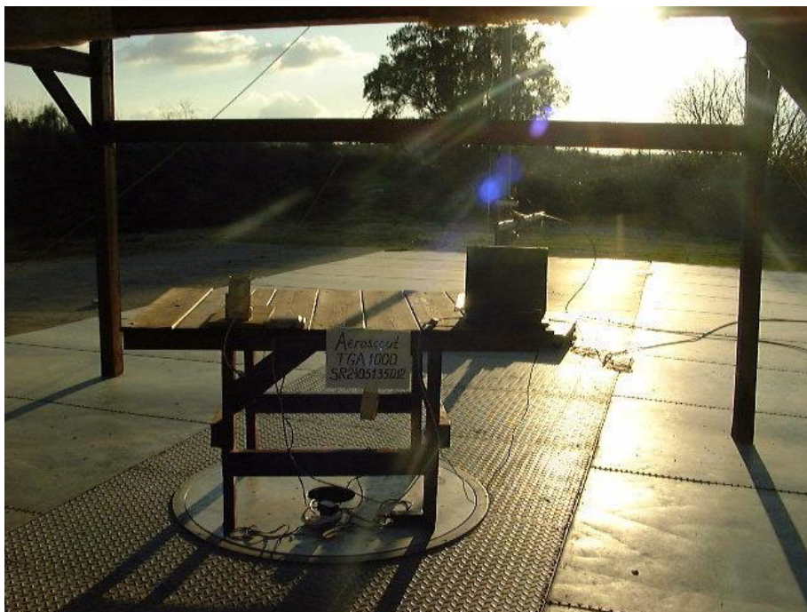
Figure 3. Spurious Radiated Emission Test Antenna SR2405135012NF
