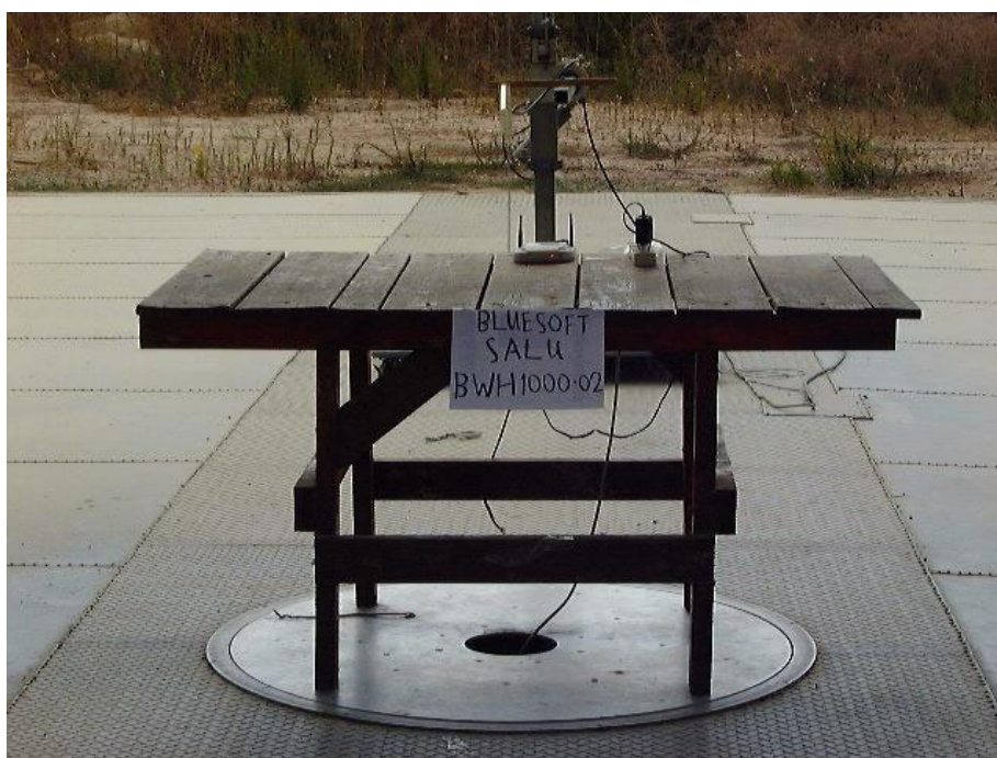
Figure 3. Spurious Radiated Emission Test Front (BWH1000-02)
