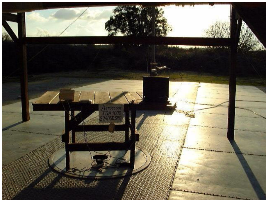
Figure 6. Spurious Radiated Emission Test Antenna S2406DSP12
