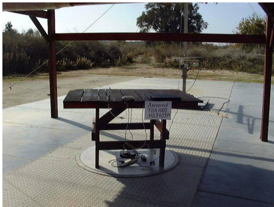
Figure 2. Spurious Radiated Emission Test Antenna HG2409P
