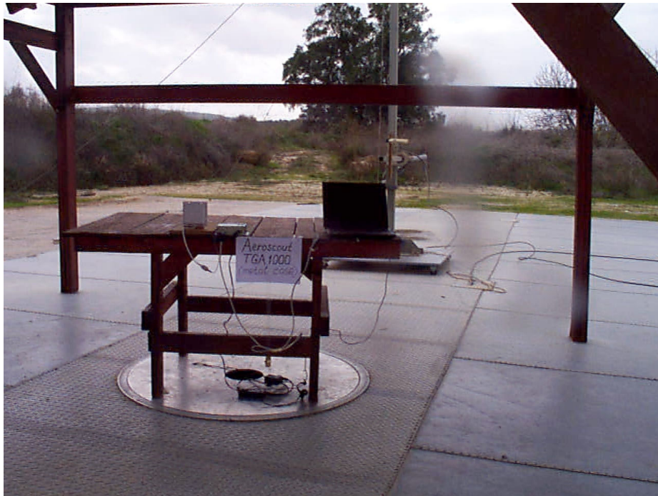
Figure 7. Spurious Radiated Emission Test Model LR-1000-R
