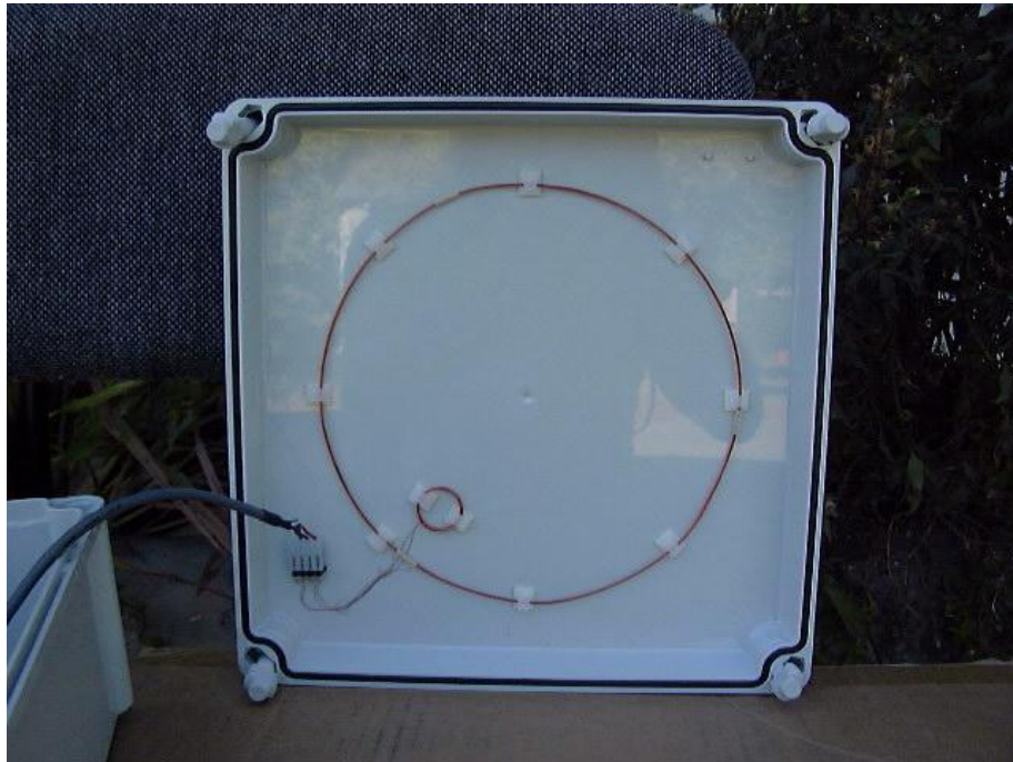
Figure 1 Front Cover Internal View With Antennas
