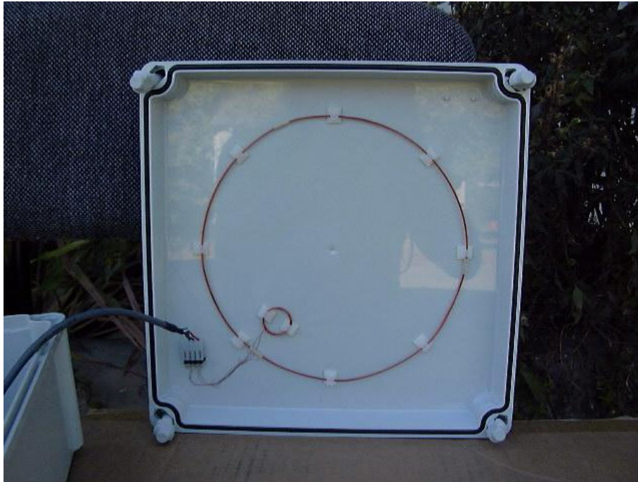
Figure 25 Front Cover Internal View With Antennas
