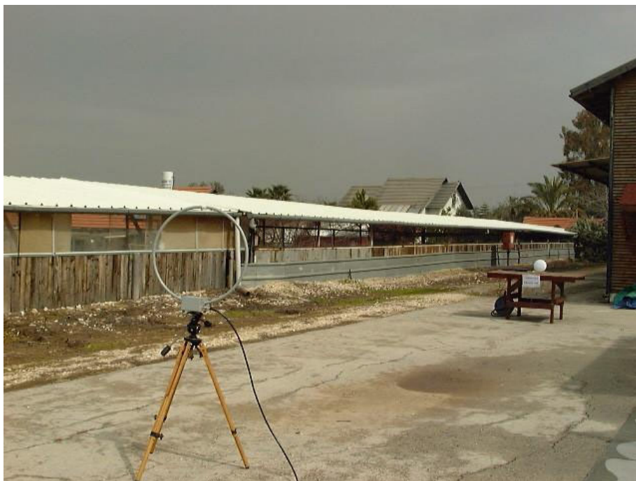
Figure 5. Radiated Emission Test 9 kHz – 30 MHz
