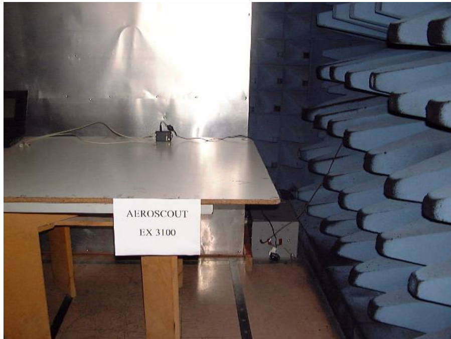
Figure 5. Conducted Emission Test.
