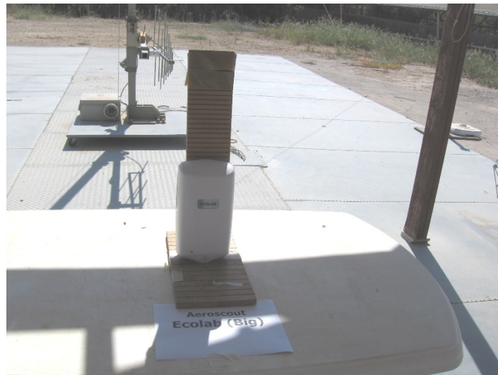
Figure 10. Radiated Emission Test M/N: 92021188 (Ecolab NEXA big)
