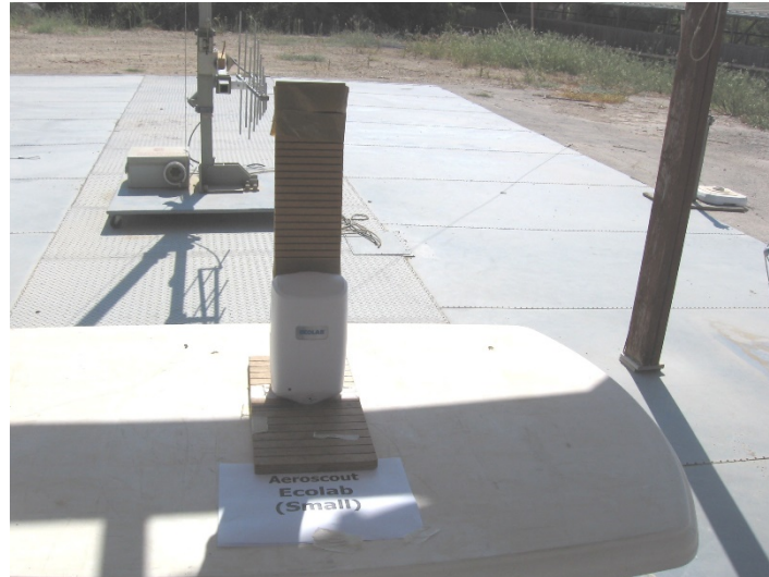
Figure 12. Radiated Emission Test M/N: 92021184 (Ecolab NEXA small)
