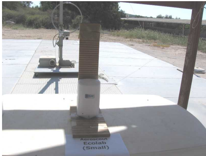
Radiated Emission Test – M/N 92021184 (Ecolab NEXA small)
