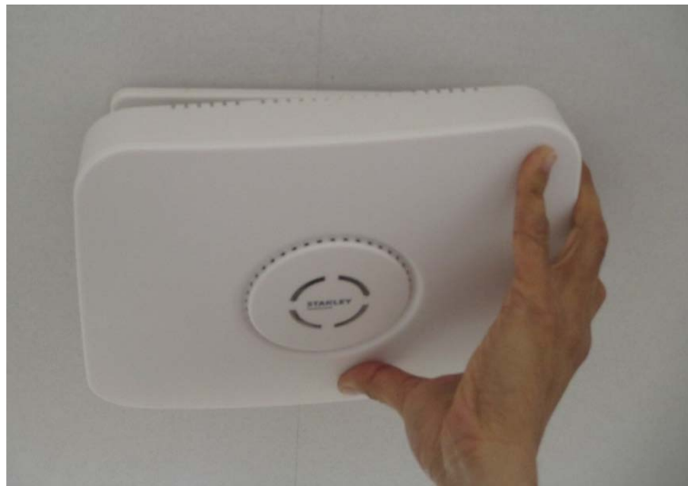
Figure 17: Attaching the Controller to the Mounting Adapter
