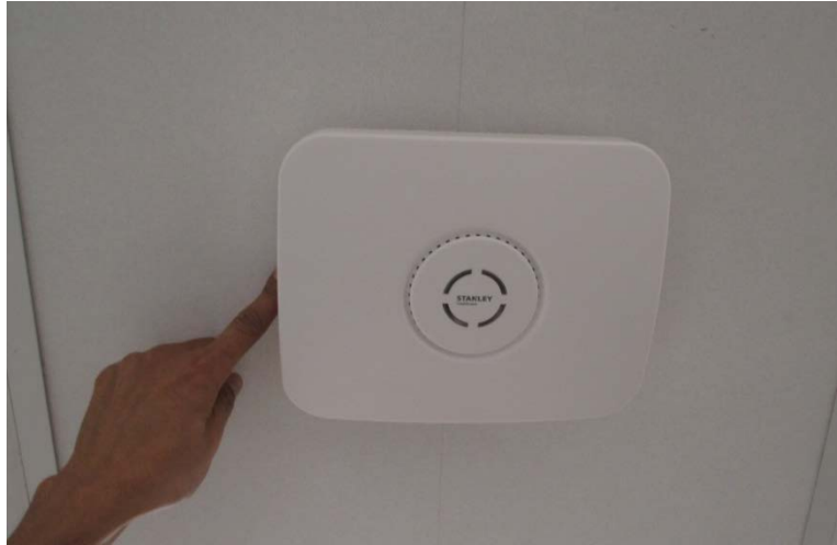
Figure 18: Releasing the Controller from the Mounting Adapter
