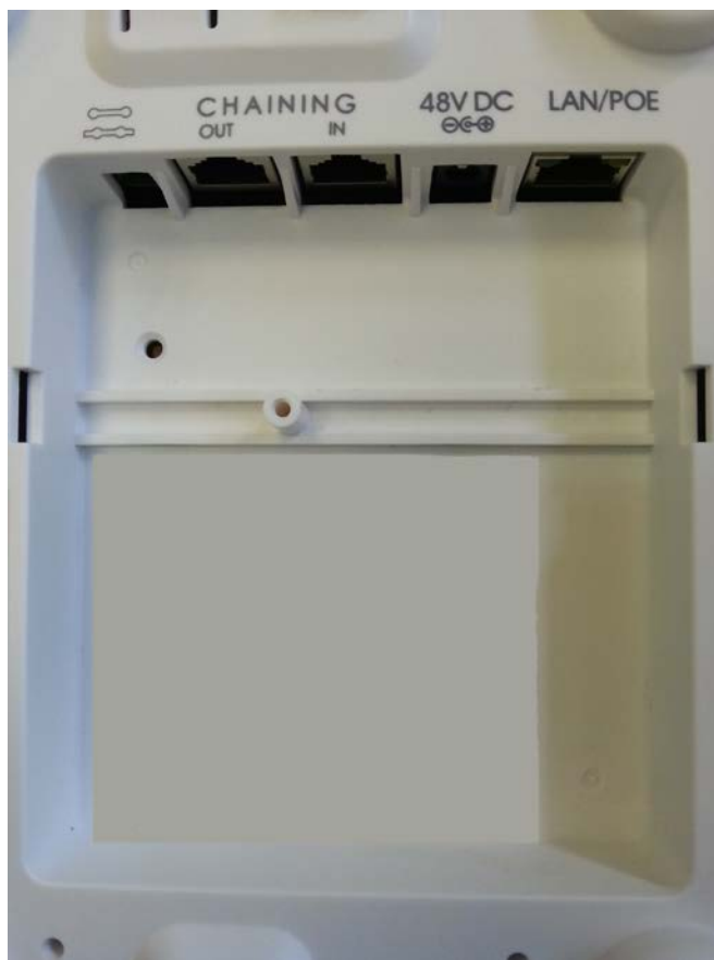
Figure 4: EX5200R Connector Wiring
