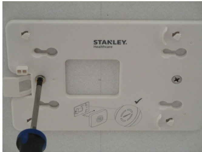
Figure 16: Screwing the Mounting Adapter to the Spacers of the Mounting Clip
