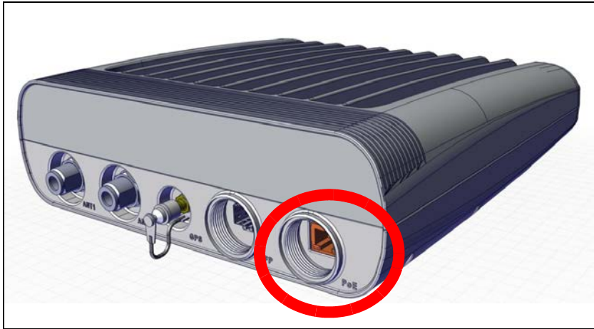
Figure 2-2: PoE port: HBS radio unit
