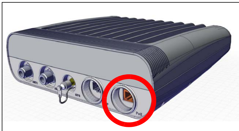
Figure 2-26: Input port: HBS unit (connection label: "PoE")
