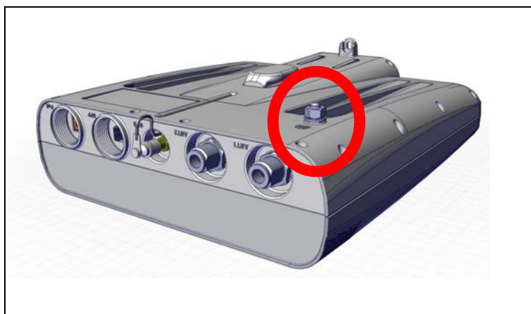
Figure 2-22: Ground: HBS radio unit
