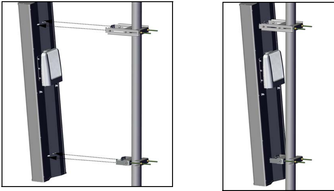
Figure 2-6: Mount HBS/ antenna on pole
