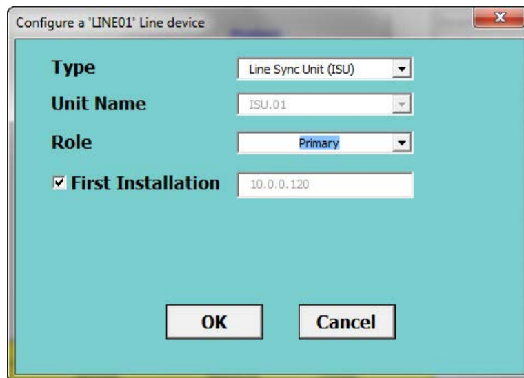
Figure 3-19: ISU - First time installation
