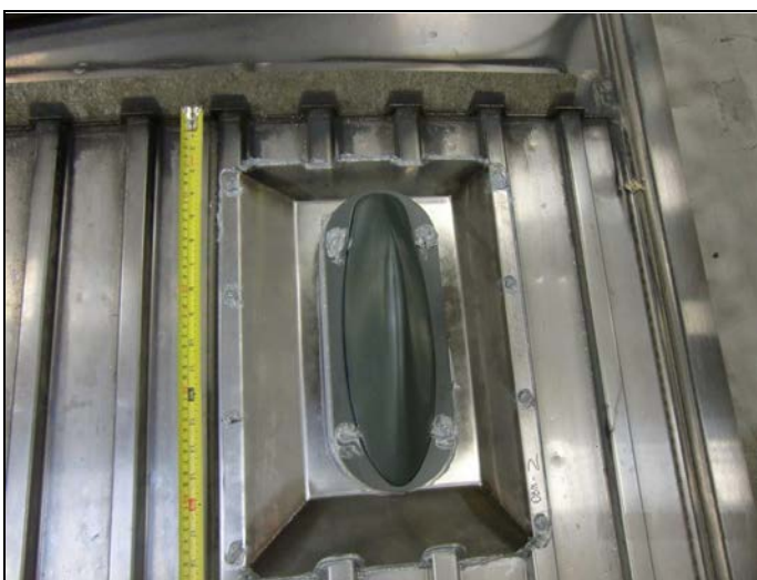
Figure 1-77: Integrated Roof Mounting Table for Shark-Fin antenna
