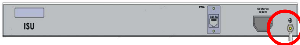
Figure 1-60: ISU: Grounding lug location
