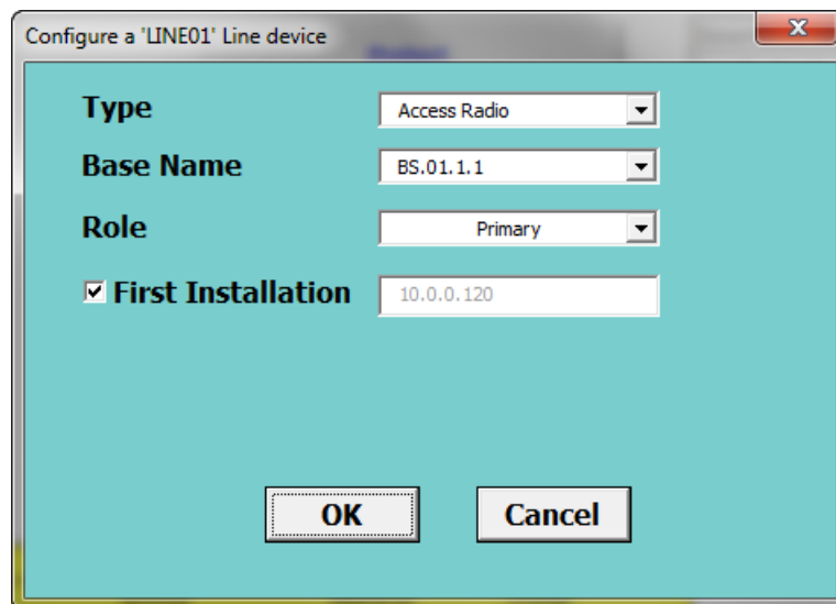
Figure 3-15: TBS - First time Installation
