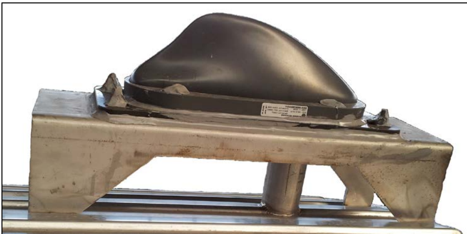
Figure 1-76: Roof Mounting Table for Shark-Fin antenna
