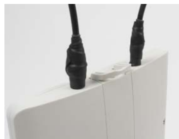
Sealing tape applied
