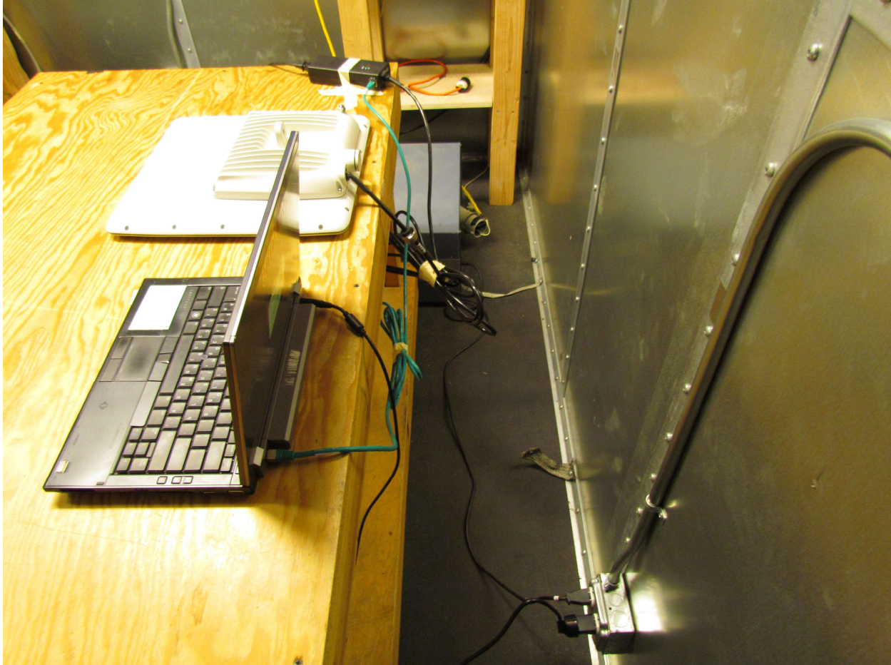
Conducted Emissions PoE configuration Side View
