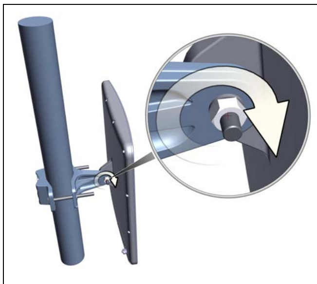
Figure 2-60: Tighten bolt (SU PRO/AIR INT shown)
