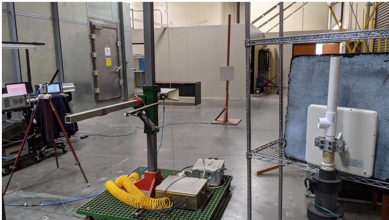
Radiated DFS Test Setup
