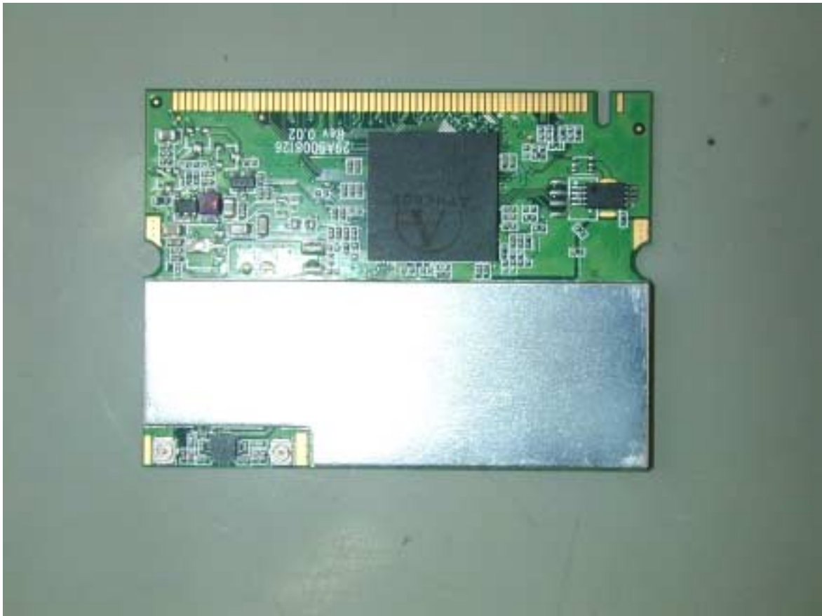
Photograph No.4 Winlink 1000/F58 and AirMux 200/F58 Modem and RF board
