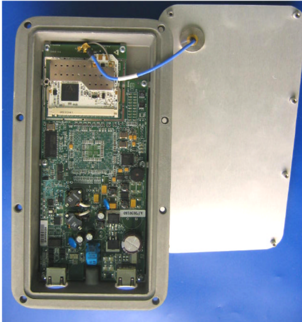
Photograph No.9 Winlink 1000-F58/HP (ODU) internal view
