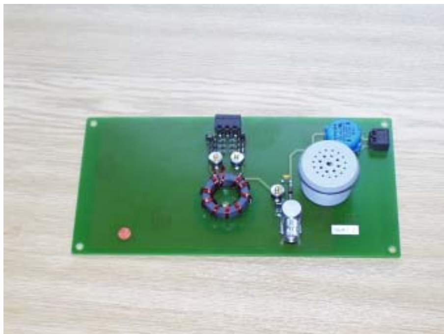
view of the PCB in the active antenna (without complementary filter)
