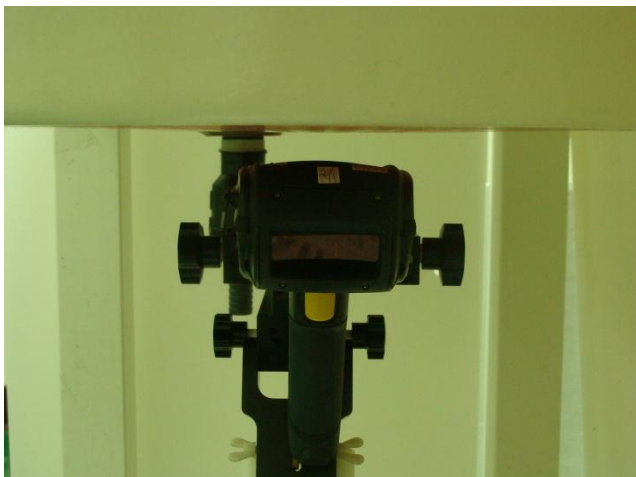
Front of the DUT with 1.5 cm Gap
