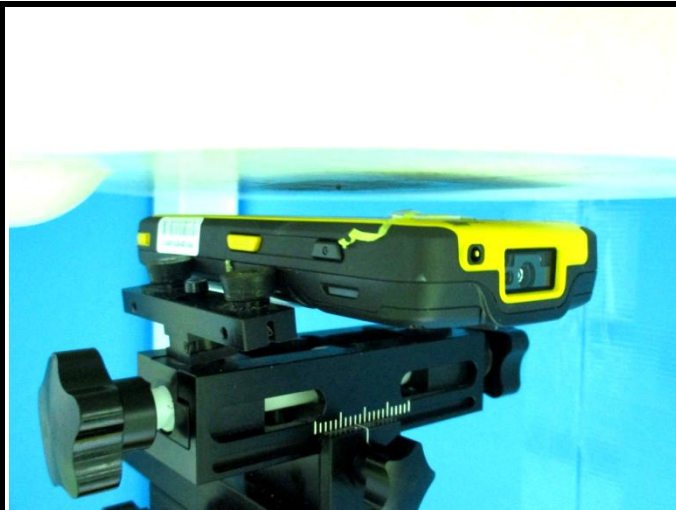
Front Face of EUT with 10 mm Gap
