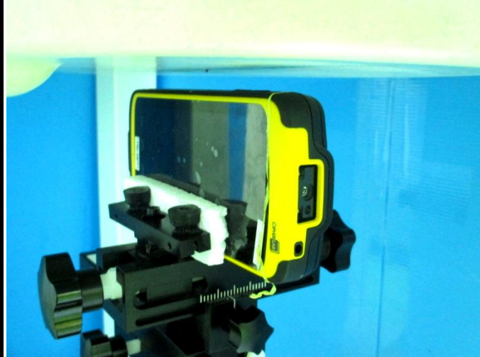
Left Side of EUT with 10 mm Gap
