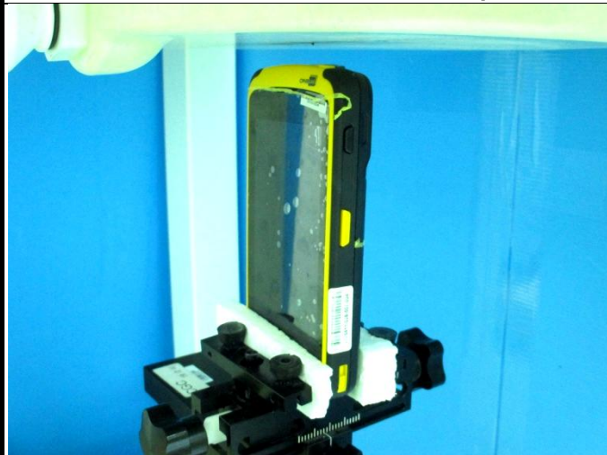
Top Side of EUT with 10 mm Gap
