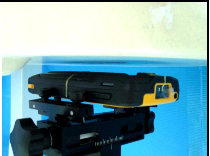
Rear Face of EUT with 10 mm Gap
