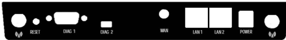
Figure 6. Motorola Cellular Gateway NC800 back panel
