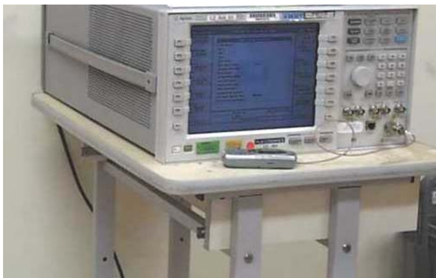
Conducted Power Measurement Setup
