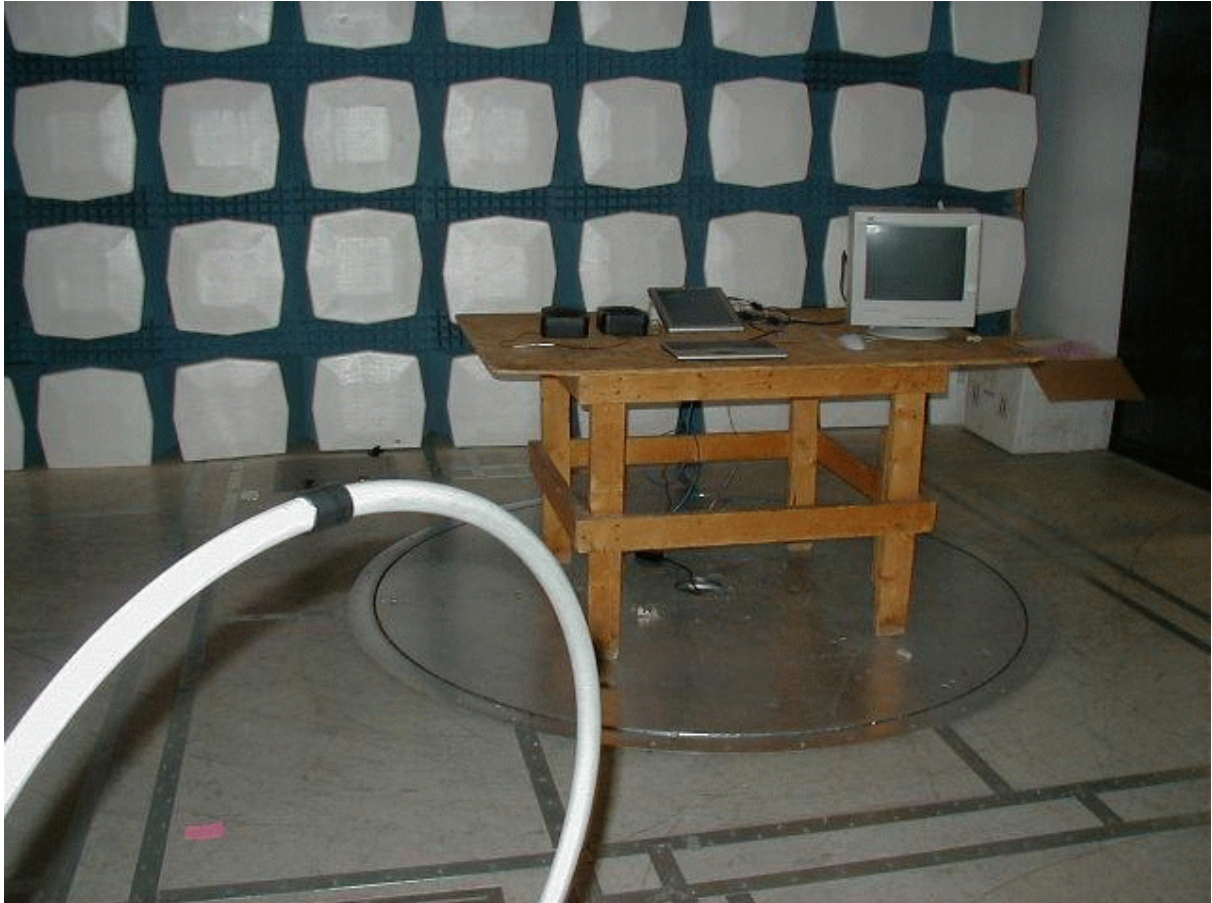
Photograph 1. FCC 15.209 Radiated Emissions Test Setup Photo
